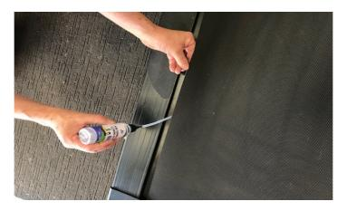
Lift up the mat and apply silicone oil onto the deck along each side, right into the middle and the complete length of the treadmill deck. For best performance and reliability ensure a good coating of silicone oil is applied to each side regularly.
