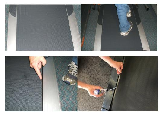
After applying silicone oil under each side of the belt, run slowly and push with feet again to centralise the belt. Run the treadmill slowly checking belt is not rubbing against the siderails.
